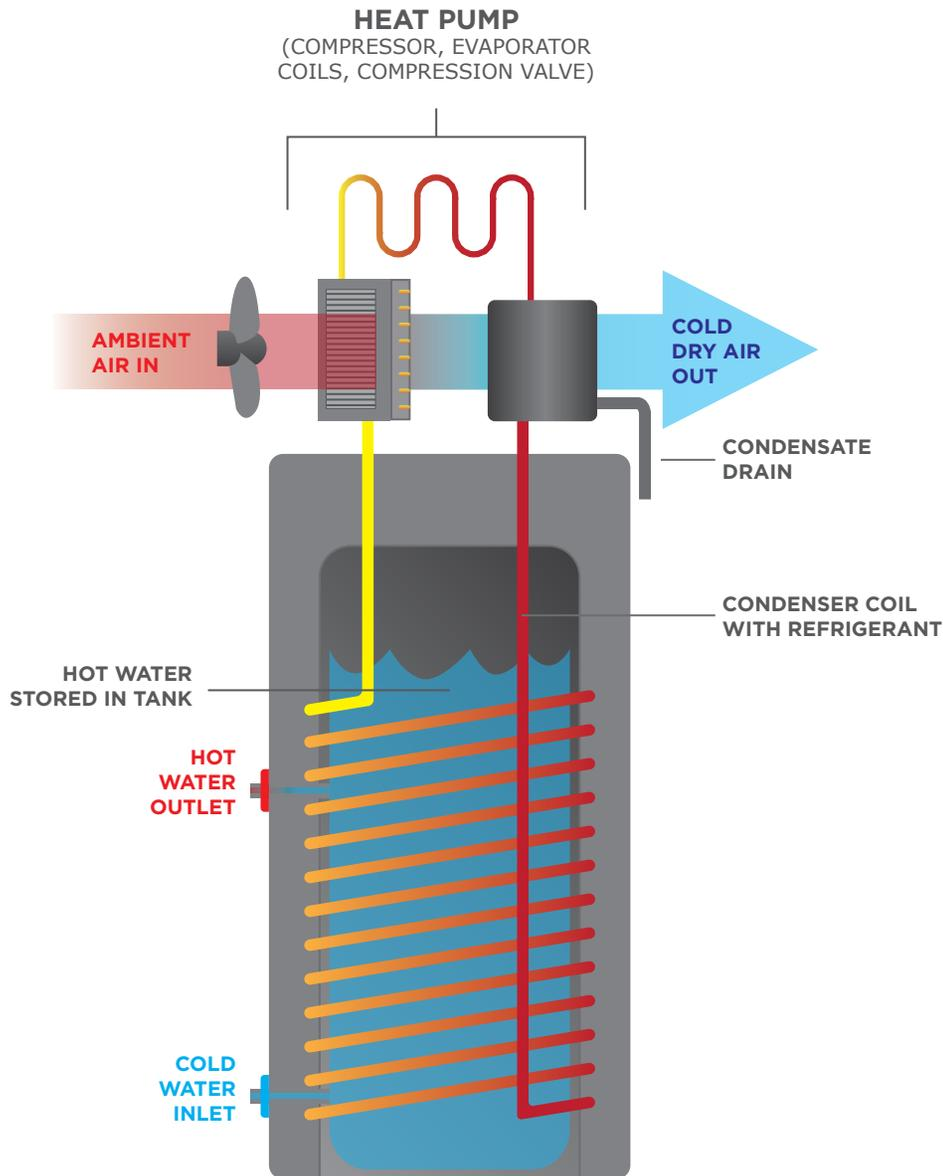
A Heat Pump Water Heater works similarly to a refrigerator, except in reverse. While a refrigerator removes heat from an enclosed box and expels that heat to the surrounding air, a HPWH takes the heat from surrounding air and transfers it to water in an enclosed tank.
